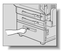
2 Pull out the paper drawer for the large-capacity paper feed cabinet.
